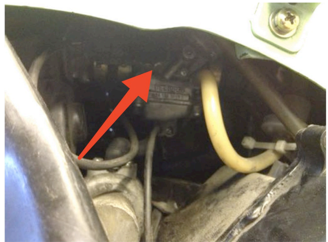
10) Adjustment to idle ( found underneath the seat ) and to carburettor air mix screw for any deadspots in the throttle range.
