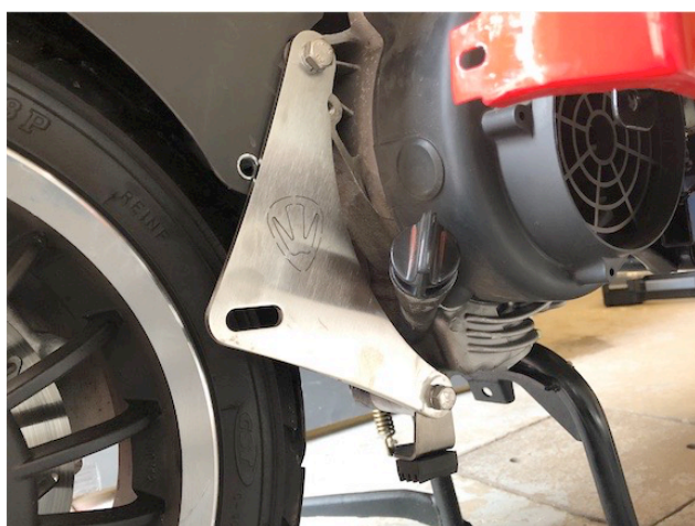
9) FIT TASSO SUPPORT BRACKET TO ENGINE
