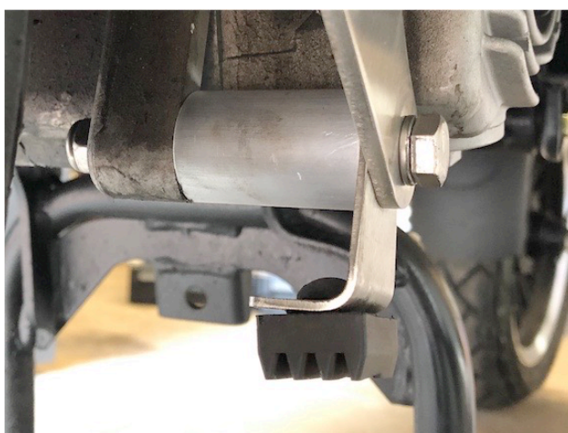
10) FIT M8 SPACER AND STAND STOP AS SHOWN
