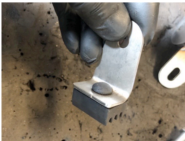
8) FIT RUBBER INTO STAND STOP BRACKET
