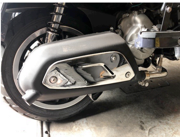
3) UNDO M8 BOLTS SUPPORTING EXHAUST.
