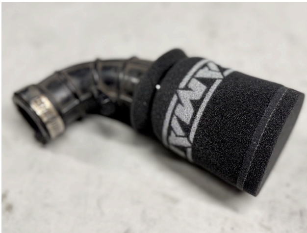
9) Remove Elbow from airbox, cut at 5 ribs and fit airsock securing with cable tie supplied
