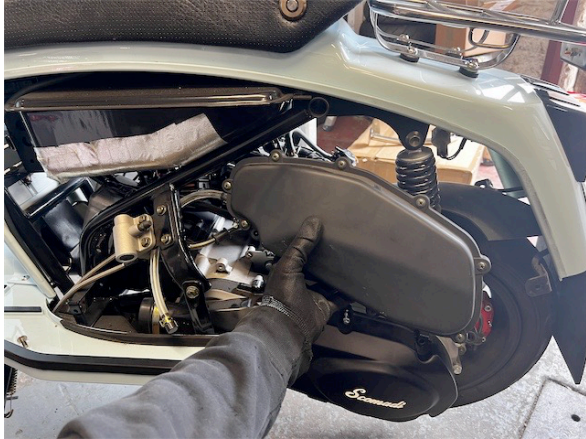
1) UNBOLT AIRBOX, DETACH BREATHER HOSES AND REMOVE.
