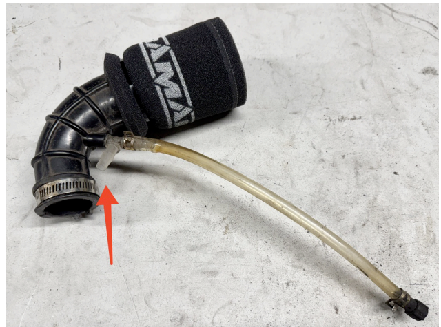
10 ) Using existing tubing assemble as shown. Arrow notes fitting of breather pipe from head to t-piece.
