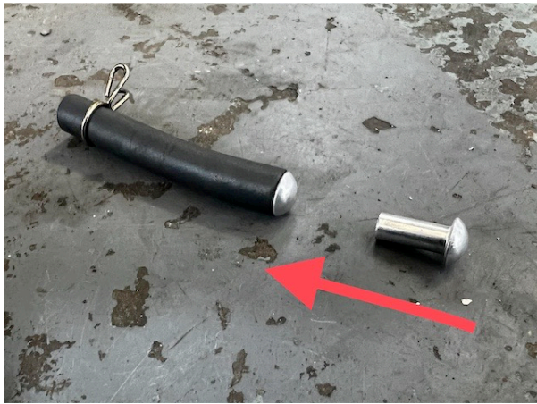
7) CUT 5cm LENGTH FROM ORIGINAL VAC PIPE AND FIT BLANK PLUG INTO HOSE END.
