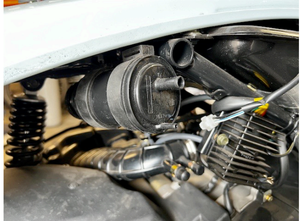
2) DETACH CHARCOAL FILTER FROM HOLDER AND REMOVE
