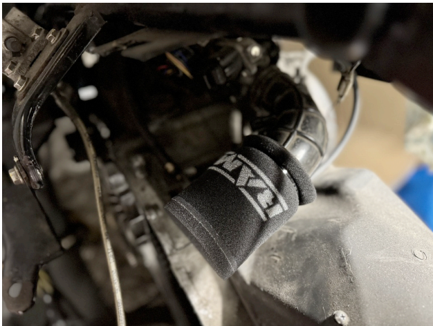
9) Remove Elbow from airbox, cut at 5 ribs and fit airsock securing with cable tie supplied
