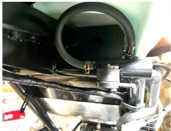
6) USING SPARE TUBE FROM AIRBOX ASSY, REFIT FUEL SHUT OFF VALVE AS ABOVE. MUST BE IN CORRECT UPRIGHT POSITION AS SHOWN
