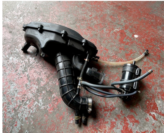
4) REMOVE AIRBOX AND CANISTER ASSY
