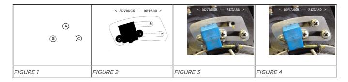
Remove flywheel cover and unscrew the pickup. On 125/150 motors, before fitting timing slider you will need to remove the flywheel. This will allow you to unclip and give free movement of the wire from the stator to the pickup. Allow an extra 10mm of wire then secure clip. On 200 motors you do not need to remove flywheel as there is enough free slack in the wire.
